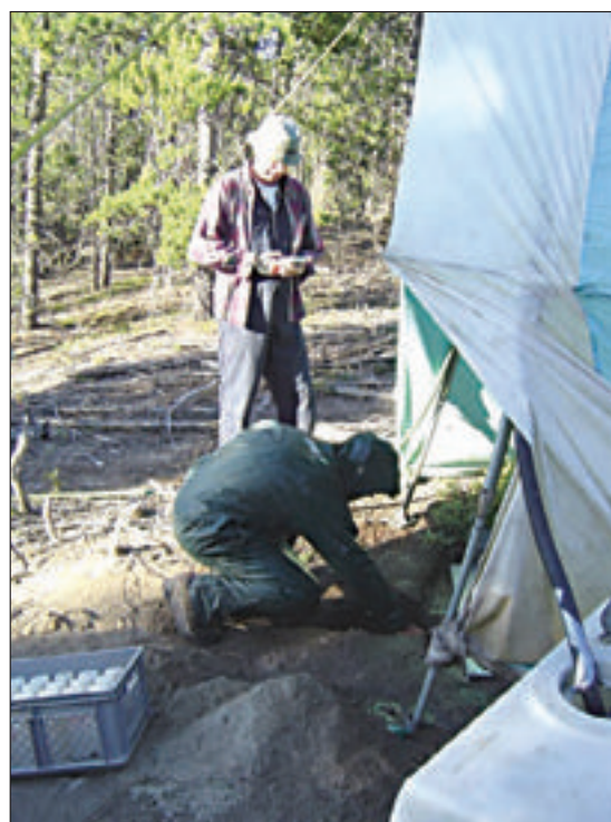
Station researchers sample runoff from a rainfall simulator to determine resource damage on an ATV trail in Montana. (photo by B. Kopyscianski)
