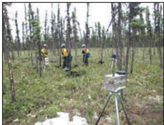
Scientists install fire-proof video cameras (background next to personnel) and fire behavior flux instruments (foreground).
