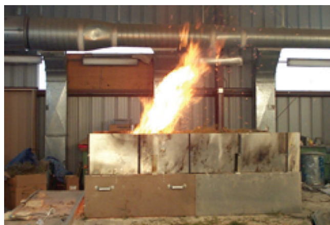
Fig. 2. A successful fire spread case in an Adenostoma fasciculatum fuel bed 40 cm deep with wind velocity of 2 \text{ m s}^{-1} and no slope.
