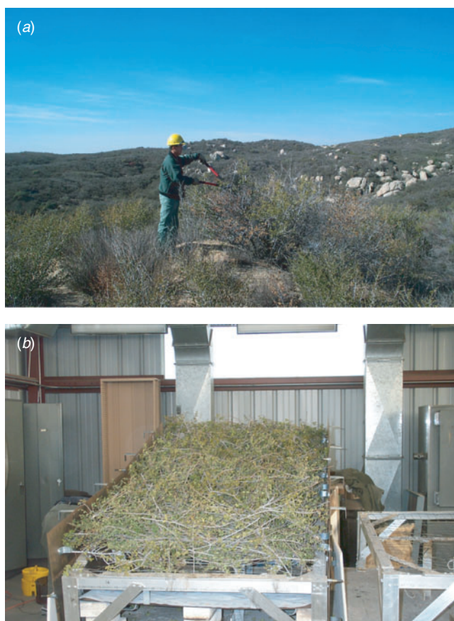
Fig. 1. (a) Fuel collection site located 50 km east of Riverside, CA, USA at an elevation of 1300 m in a mixed chaparral stand. Shrubs are young Ceanothus crassifolius . (b) Fuel bed constructed of live foliage and branches <0.64 cm diameter of C. crassifolius .
