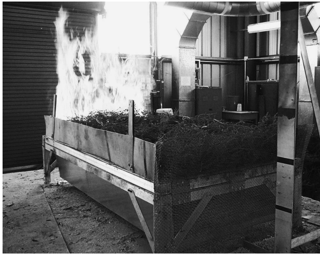
Fig. 3. Experimental setup of the fuel bed constructed of live foliage and branches of chamise with 2.0 m long, 1.0 m wide, and 0.2 m deep. The fire illustrates the initial ignition, and the ruler at the right side shows the scale with 0.25 m.
