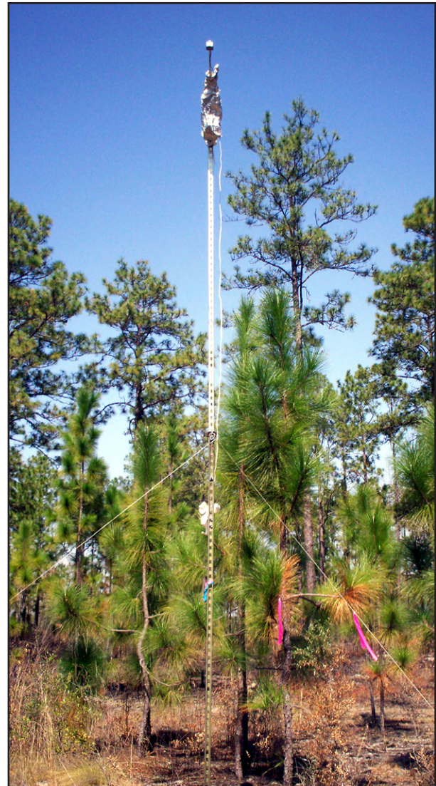
Figure 2. Overhead fire monitoring station for field use consisting of a downward-pointing dual-band infrared sensor, weather and gas ( \text{CO} , \text{CO}_2 ) sensors, all mounted on a portable 6.2 m tower. The image was captured during a series of experiments (Rx-CADRE) conducted in the longleaf pine-wiregrass ecosystem of the southeastern United States.
