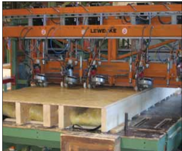
Figure GD9. LeWecke machine nailing panels onto roof section.
