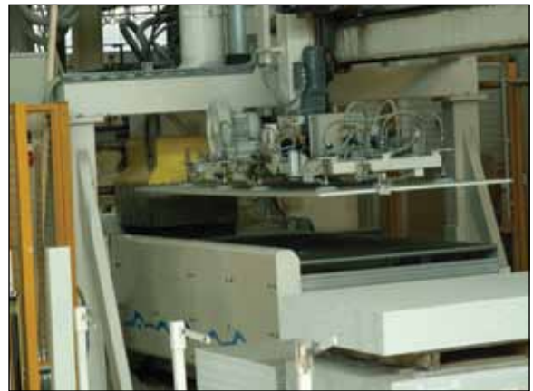
Figure GG5. Weinmann panel processor cuts 150 thousand sheets per year.
