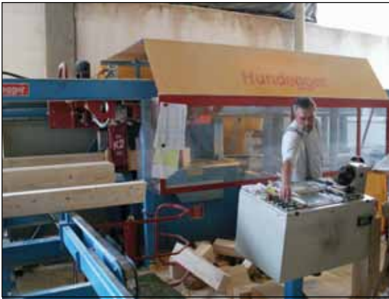
Figure GH2. Newer Hundegger beam processor used for floor and roof components.
