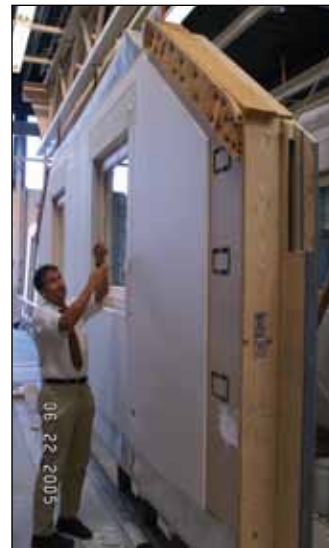
Figure GG11. Wall section hung vertically: Note cut out areas used to connect adjacent walls at building site.
