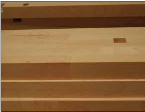
Figure GF4. Edge-glued and fingerjointed beech panels were common stock for stairs.
