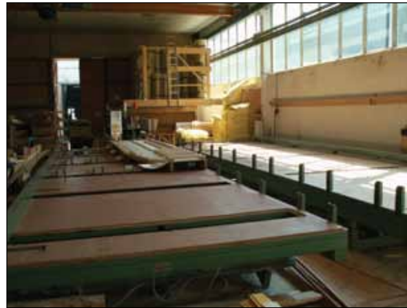
Figure GH4. Tables used in the ceiling and roof building area.
