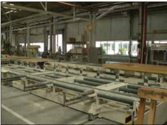
Figure GE6. Butterfly table used to flip wall panels as they move down the line (background).
