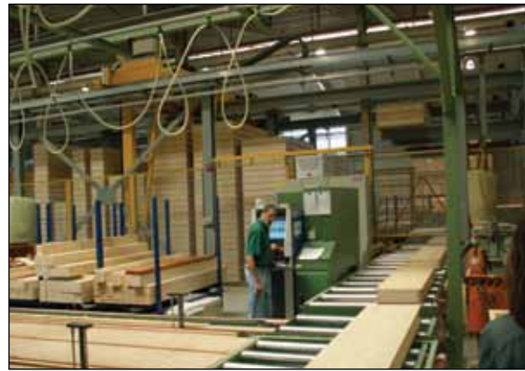
Figure GD2. Staging area into which wall panel elements are correctly sequenced.
