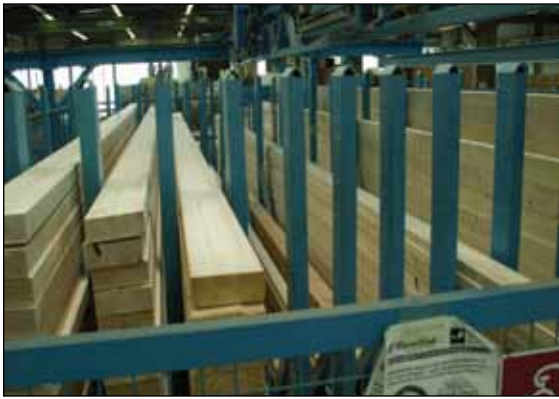
Figure GA6. Weinmann automated timber loader selected and picked up timbers from the infeed bays using screws.
