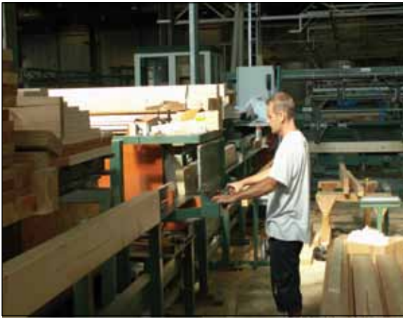
Figure GG7. Burmeck wall machine requires many manual actions.
