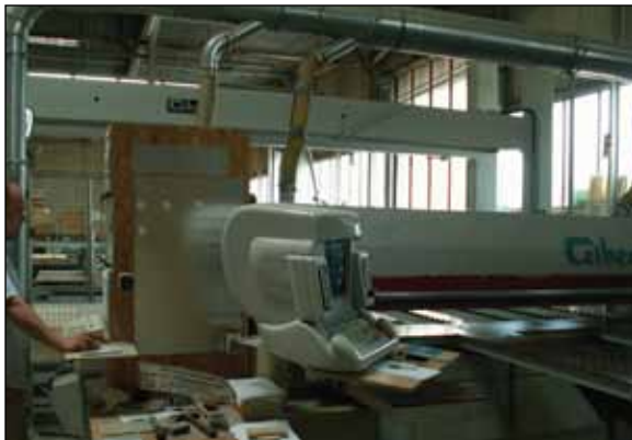
Figure GA8. Large Giben computer numerical controlled (CNC) panel processor cut oriented strandboard (OSB), particleboard, and plywood.
