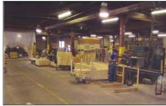
Figure F9. Component plant produced rafters, doors, doorframes, cut countertops, and inventoried purchased items such as cabinets, commodes, sinks, insulation, and flooring.
