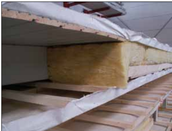
Figure GF11. Stacked roof sections with insulation.
