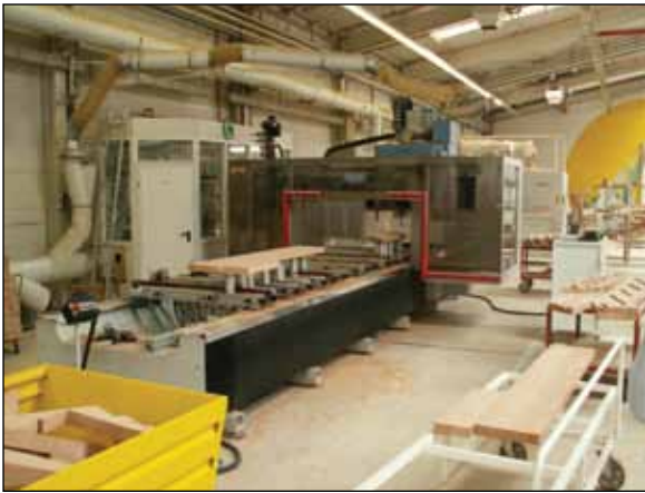
Figure GE11. Maka CNC machine used vacuum pods to hold stock used to produce beech stair parts.
