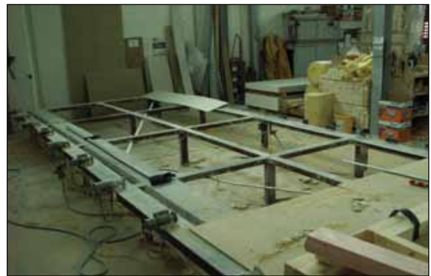
Figure GC3. Frame table with air-activated cylinders to clamp and hold frame.
