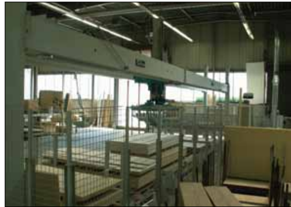
Figure GA9. Giben infeed with many panels available for vacuum lift.
