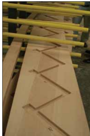
Figure GA23. Beech stair stringer machined with computer numerically controlled (CNC) router.
