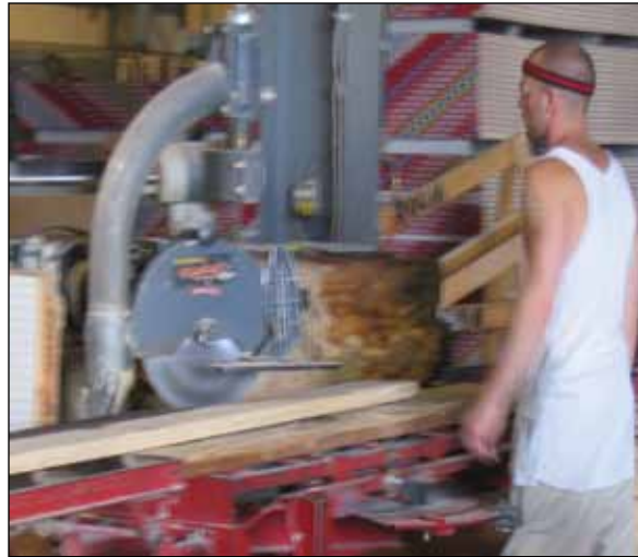
Figure D3. In the mill room, chop saw used to cut different angles on rafters.
