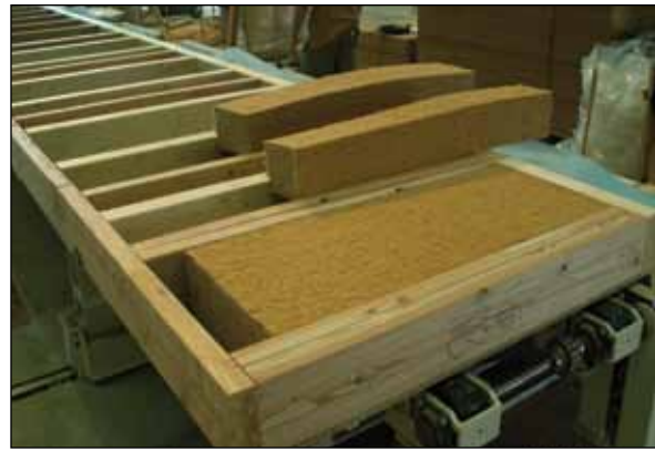
Figure GG10. New wood-based (5% polyethelene) insulation.
