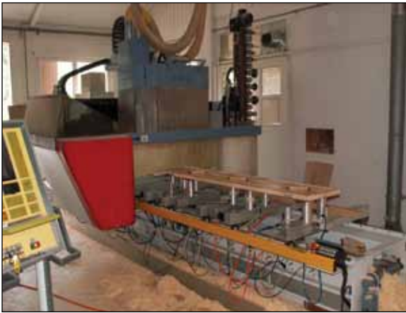
Figure GF3. Maku computer-numerical-controlled (CNC) router used to machine door and stair components.
