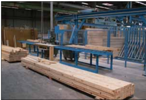
Figure GA7. Manual cut-off saw used for short timbers (infeed bays for the Hundegger shown in background).
