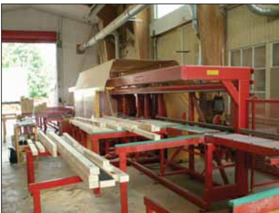
Figure GF5. Hundegger computer-numerical-controlled (CNC) timber processor used for wall components.
