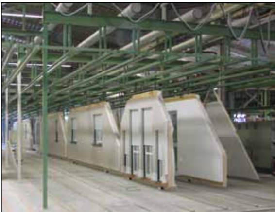
Figure GD7. Wall sections hung on vertical storage racks.
