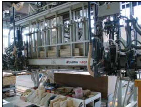
Figure GG12. Older model Weinmann multifunction bridge lays and nails furring strips.
