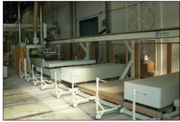
Figure GG4. Weinmann panel processor cuts gypsum and particleboard panels.
