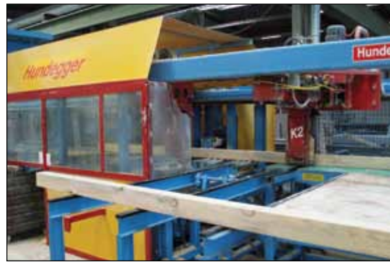
Figure GA3. Shielded sawing and notching area of the Hundegger K2. The red clamps are feeding a timber to the cutting heads.
