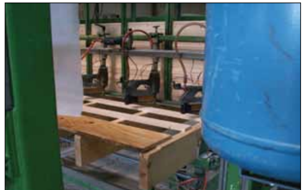
Figure GA17. Automatic board dealer and automatic nail gun fastens furring strips to joists at the middle floor station (floor and ceiling).
