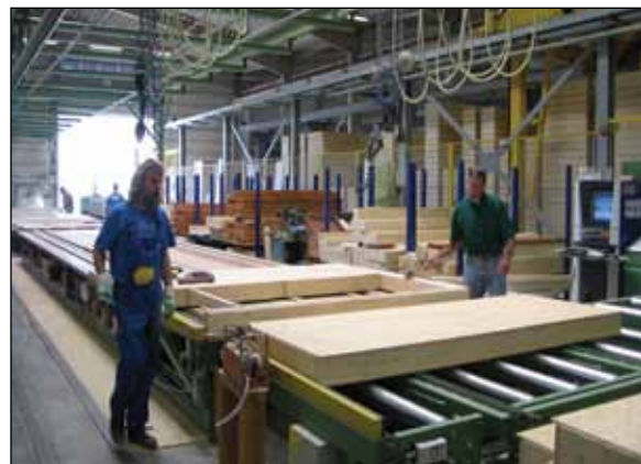
Figure GD3. Assembly table workers manually connecting standardized elements together.
