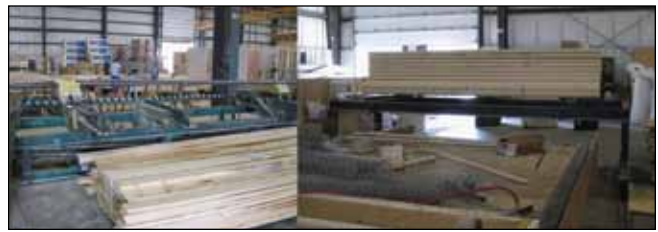
Figure D2. Precision end trim (PET) saw used to trim lengths (left) and joist dealer carriage (right).
