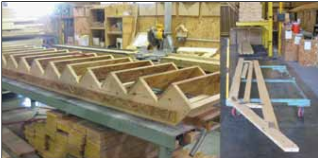
Figure B1. Plant B built its staircases and roof trusses in-house.
