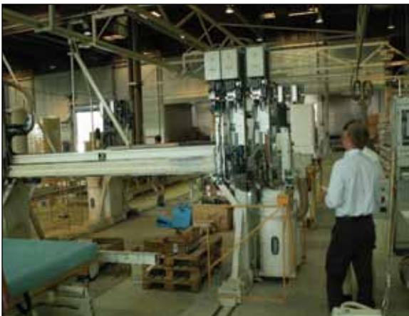
Figure GG9. Automated stapler is used to fasten moisture barrier.
