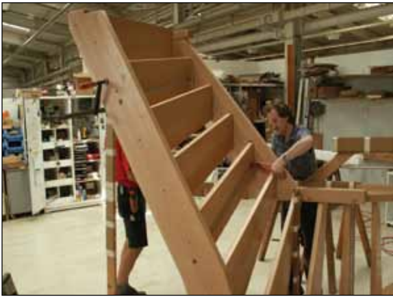
Figure GE12. Staircase assembly.
