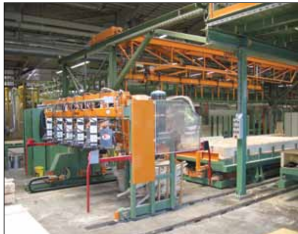
Figure GD10. View of LeWecke machine capable of dealing lathe and automatic nailing.
