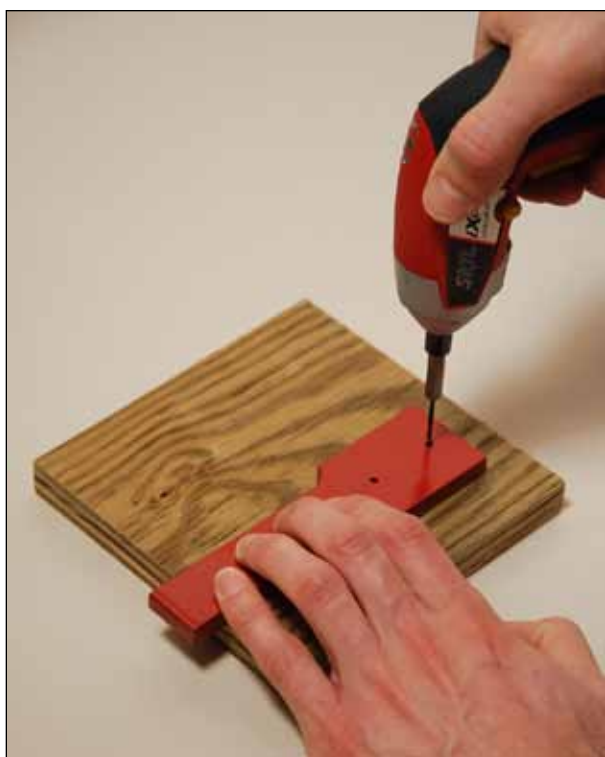
Figure 2—ACQ-treated plywood specimen and template used for pre-drilling pairs of holes.
