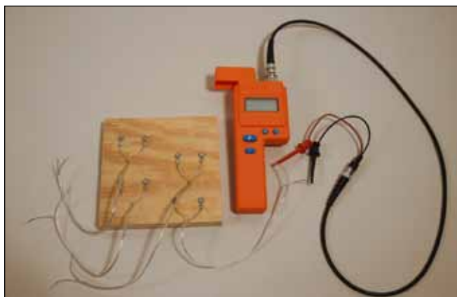
Figure 1—Experimental set-up for moisture meter readings: untreated plywood specimen, stainless steel screw electrodes with leads, moisture meter, and cable assembly with mini hook clips. In the specimen shown, the unsanded surface is sapwood and contains no defects.
