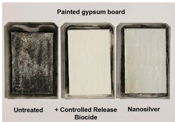
Figure 2. Painted gypsum board demonstrates effectiveness of controlled release nano-carrier following challenge with Aspergillus niger . Untreated control (left); treated with nanotubules loaded with commercial biocide (center); treated with nanotubules loaded with nanosilver (right).
