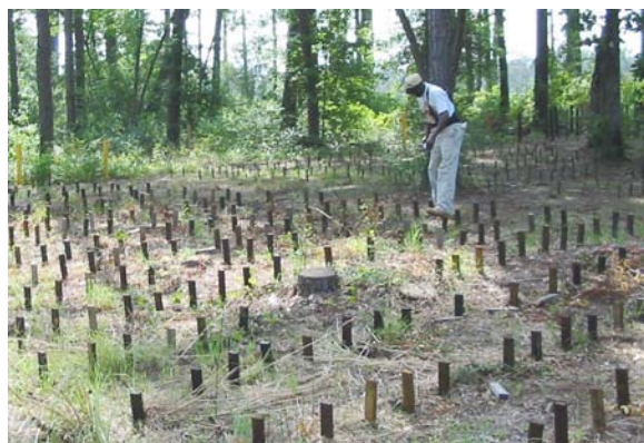
Figure 2. Stake test plot in Mississippi, USA.
