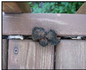
Figure 5. Current above-ground test methods may not adequately account for the accumulation of organic debris that can occur in-service.
