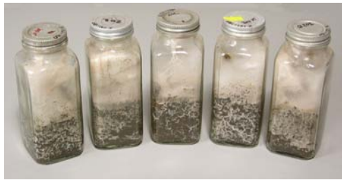
Figure 1. Soil block (or soil-bottle) decay test.
