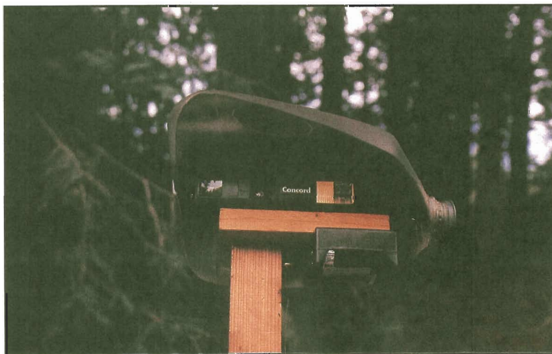
Figure 6 —Line-triggered camera station. Protective milk jug in place.
