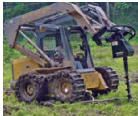
Figure 7.6.20 —Augers are effective planting tools because one skilled operator can create planting holes (A&B) and several other workers plant the stock (C) and fill the holes by hand (D). Tractor-mounted augers can create holes large enough for the biggest container stock (E).
