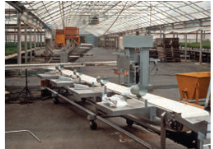
Figure 7.3.8 —Each grading station in the “pull and wrap” operation has a rack to secure the containers (A). In larger nurseries, grading stations are part of grading and packing lines, which increase efficiency (B). Because plants are often difficult to pull from containers, such as the Styroblock™, they are first run through a “thumper” that loosens the plugs (C). If roots have formed a mat at the drainage hole (D), they must be trimmed to ease extraction (E).
