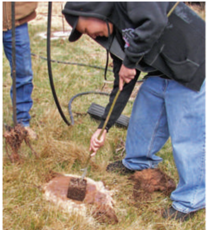
Figure 7.6.24 —The pot planter uses high-pressure water pumped from a compressor (A) through holes in a specialized nozzle (B) to create planting holes for large container stock (C).
