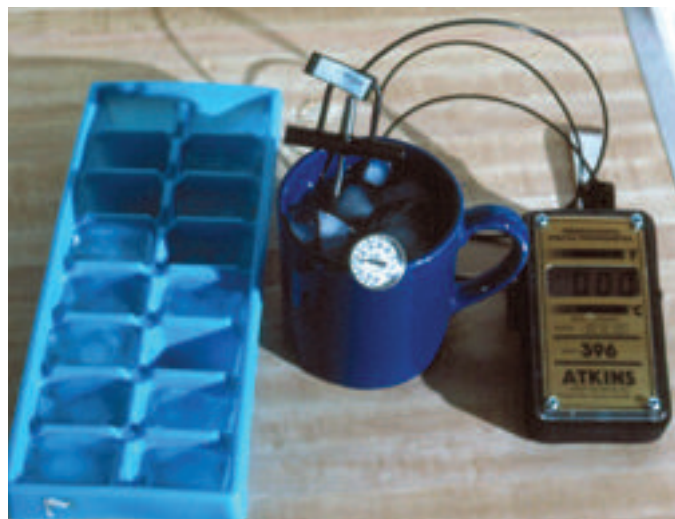
Figure 7.4.16 —Temperature can be monitored with long-stemmed electronic thermometers (A). Small hygrothermographs like the Datalogger® can monitor both temperature and relative humidity (B). Even smaller, the iButton® can monitor temperature for weeks or months, and the data can be downloaded to a computer (C). Calibrate any thermometer in a water and ice mixture to make sure it is accurate (D).
