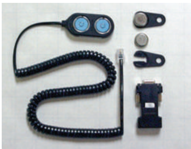
Figure 7.4.16 —Temperature can be monitored with long-stemmed electronic thermometers (A). Small hygrothermographs like the Datalogger® can monitor both temperature and relative humidity (B). Even smaller, the iButton® can monitor temperature for weeks or months, and the data can be downloaded to a computer (C). Calibrate any thermometer in a water and ice mixture to make sure it is accurate (D).
