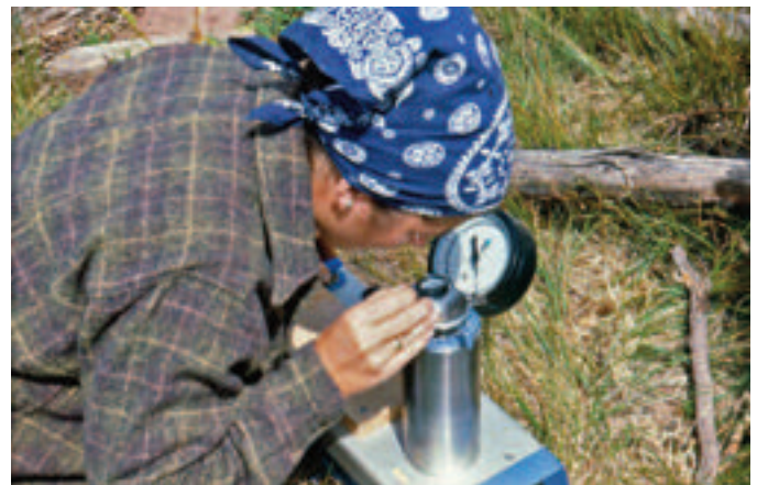
Figure 7.6.3— Nursery stock should be inspected upon delivery to the outplanting site. Check in-box temperatures of boxed plants (A) and, if possible, measure the plant moisture stress with a pressure chamber (B). Storage molds can become a serious problem in onsite storage, so check for gray or colored mycelia within the foliage (C).
