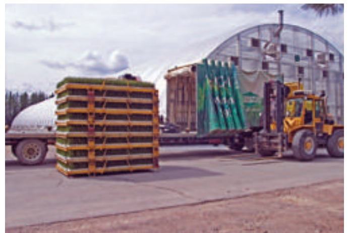
Figure 7.5.8 —Shipping plants in their growth containers requires a rack system to support and protect the stock (A). One drawback of this system is that containers must be returned to the nursery and can be damaged in transit (B). Some large forest nurseries have developed sophisticated rack handling systems for shipping plants to the outplanting site and returning the used containers to the nursery (C&D). One advantage of shipping in the growth container is that plants can be irrigated prior to outplanting (E) (C&D, courtesy of J.D. Irving, Limited).
