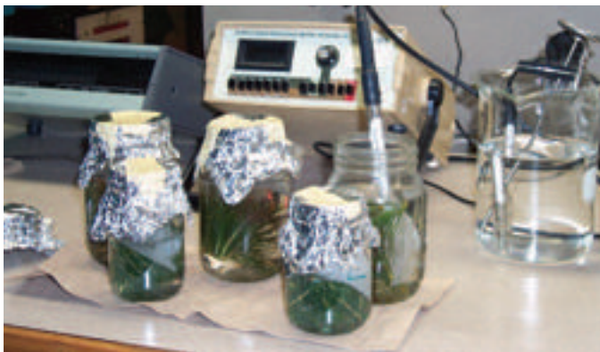
Figure 7.2.18 —In the freeze-induced electrolyte leakage test, plant tissue samples (A) are exposed to freezing temperatures (B) and then immersed in deionized water. The relative increase in electrical conductivity is an indication of cold injury (C) (C, courtesy of Sonia Gellert).
