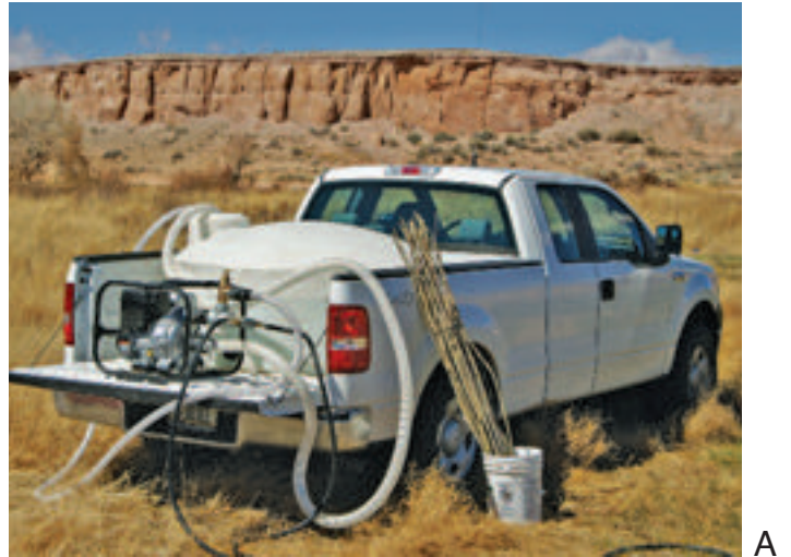
Figure 7.6.24 —The pot planter uses high-pressure water pumped from a compressor (A) through holes in a specialized nozzle (B) to create planting holes for large container stock (C).
