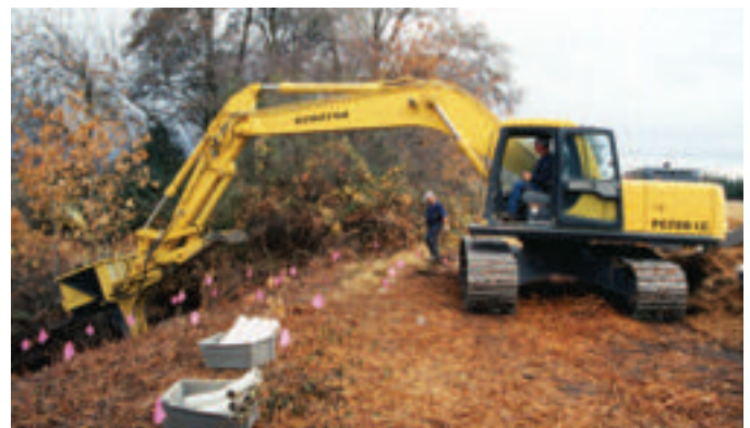
Figure 7.1.8 —The type of outplanting tool has a significant effect on the target plant. Hand-planting tools, such as the Pottiputki (A), were developed to handle paperpot seedlings, one specific type of container stock. With mechanical planting machines (B), plants must be grown in a particular size and shape to fit the handling system. The special stocktypes needed for restoration projects require innovative new outplanting equipment, such as the Expanded Stinger, which was developed for tall pots (C).
