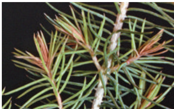
Figure 7.2.17 —In the whole plant freezing test, plants are exposed to cold temperatures in a chest freezer (A) with programmable capabilities (B). After a specified exposure period, plant tissues are rated for “browning” of buds (C), foliage (D), and lateral cambium (E).
