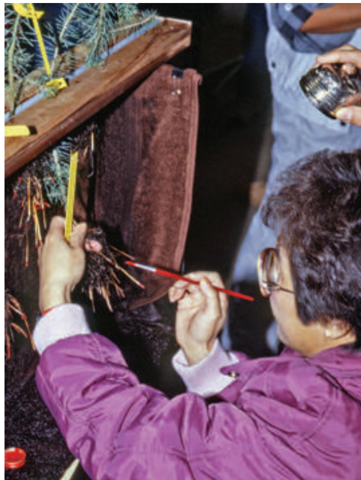
Figure 7.2.40 —Because the relationship between new roots and outplanting success is intuitively important (A), the root growth potential test quickly became the most popular and widely used assessment of plant quality. One testing procedure involves growing test plants in pots in a greenhouse (B), washing roots (C), and then rating the amount of new root growth. In the second procedure, test plants are supported in a mist chamber (D) and then measured for the length and number of new roots (E).
