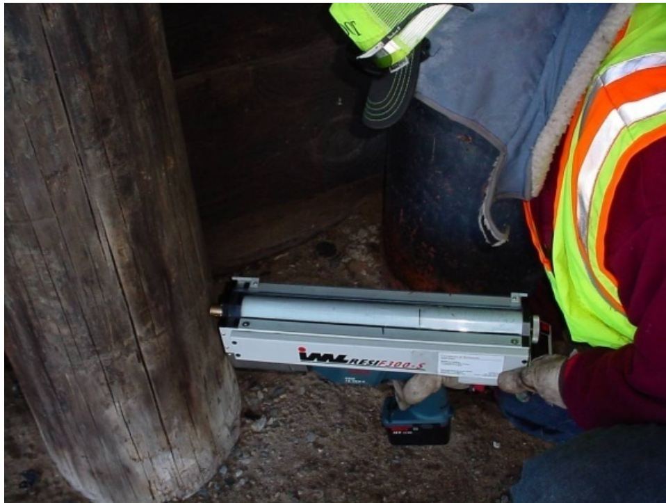
Figure 3.2. Example of resistance drill testing.
