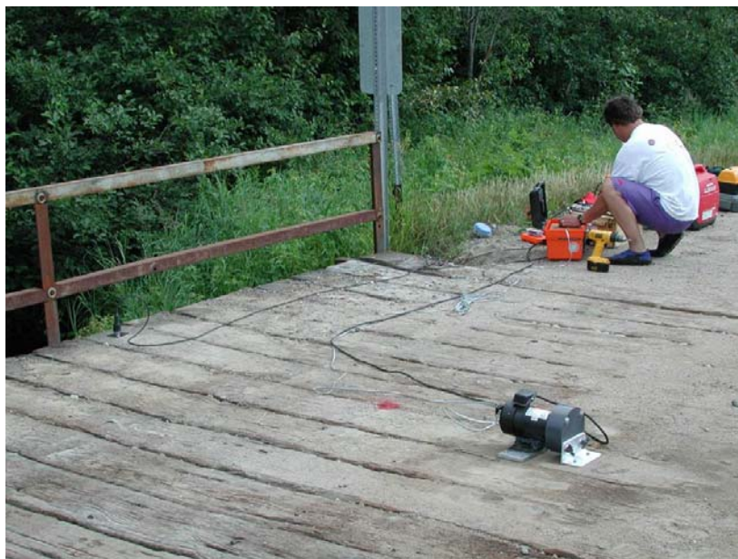
Figure 3.3. General test setup for vibration testing.
