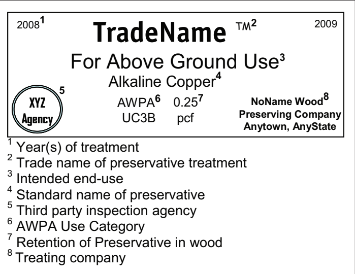
Figure 22. Grade mark stamp of preservative-treated wood. (1) The identifying symbol, logo or name of the accredited agency. (2) The applicable American Wood Preservers' Association (AWPA) commodity standard. (3) The year of treatment if required by AWPA standard. (4) The preservative used, which may be abbreviated. (5) The preservative retention. (6) The exposure category (Above ground, Ground contact, etc.). (7) The plant name and location, or plant name and number, or plant number. (8) If applicable, moisture content after treatment. (9) If applicable, length and class. (Source: Forest Products Society)
