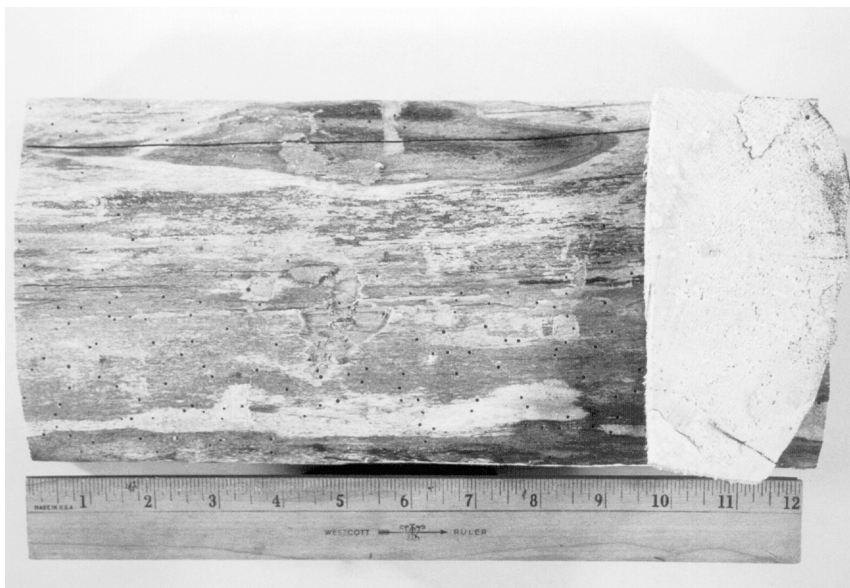
Figure 14. Anobiid beetle exit holes are round and vary in diameter from 1/16 inch to 1/8 inch. Zone lines on the end grain also indicate wood decay is present. (Source: Forest Products Society)
