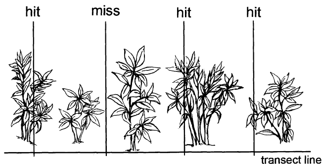
Fig. 5.2 The point-intercept method tallies vegetation hits touching a pole perpendicular to a transect at predetermined intervals
