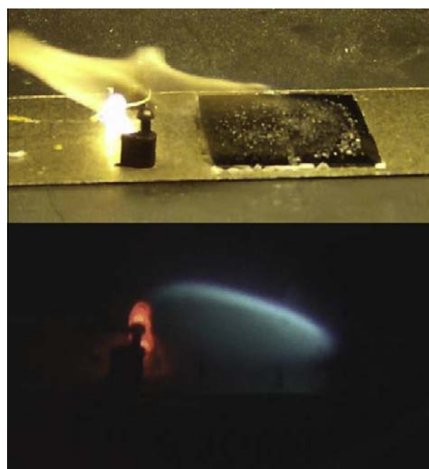
Fig. 4. Photographs of the flames in air at atmospheric pressure (above) and at 27.6 kPa (below).
