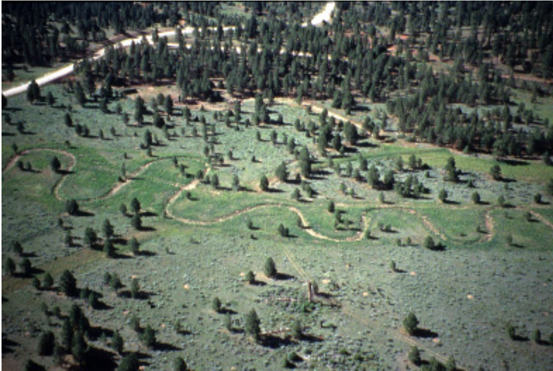
Figure 1 —This photo shows the “green belt” surrounding the meanders of the newly installed channel. This channel is shallow and wide with 37 meanders in the study area. The old channel show in figure 1 is relatively straight and more deeply incised.
