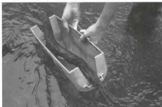
FIGURE 2. Longitudinal sieve sampler (45 cm long) for retrieving snags up to 8 cm in diameter. The sampler is placed under snag before it is pulled out of the water. Excess wood is clipped or sawed off each end, and the remaining piece is placed in a plastic bag, along with any invertebrates that dropped into the sieve.
