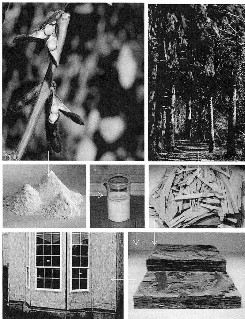
Fig. 1. Conversion of plants to houses. The left side illustrates the conversion of the soybeans to flour and then to liquid adhesive, which is used to bond the strands that come from the trees shown on the right side. The strands and adhesive make strandboard used in housing construction.
