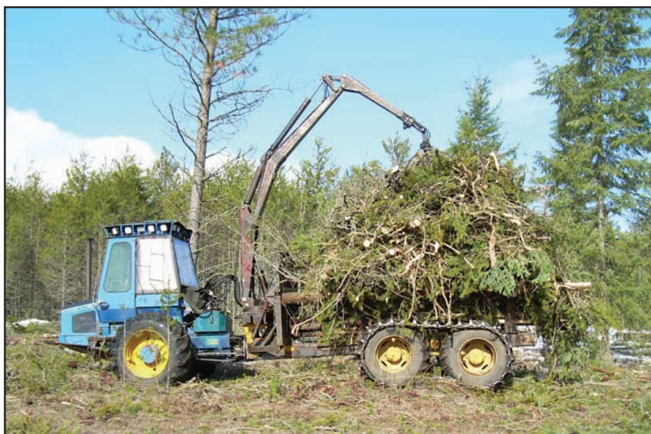
Figure 2 —Loose slash transported from harvest area on a small-scale forwarder.
