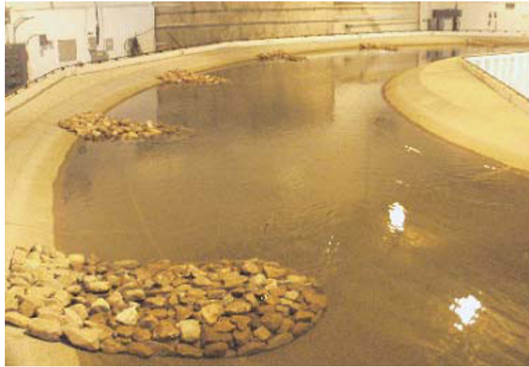
Figure 3. Bendway weirs installed in model channel. This figure is available in colour online at wileyonlinelibrary.com
