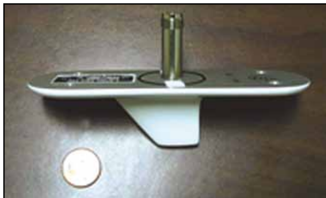
Figure 5— View of the aircraft gain blade antenna that is attached to the aircraft's fuselage.
