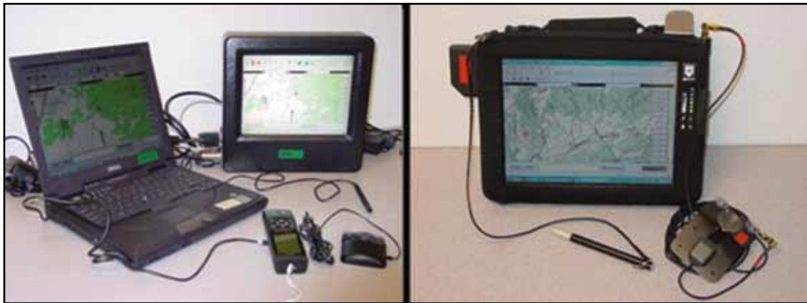
Figure 2—Forest Service digital sketchmapping systems are displayed. At left is the two-screen system with external global positioning system (GPS) receiver. At right is the pen-tablet sketchmapping table with built-in GPS receiver (the windshield-mounted antenna is shown in the lower right).
