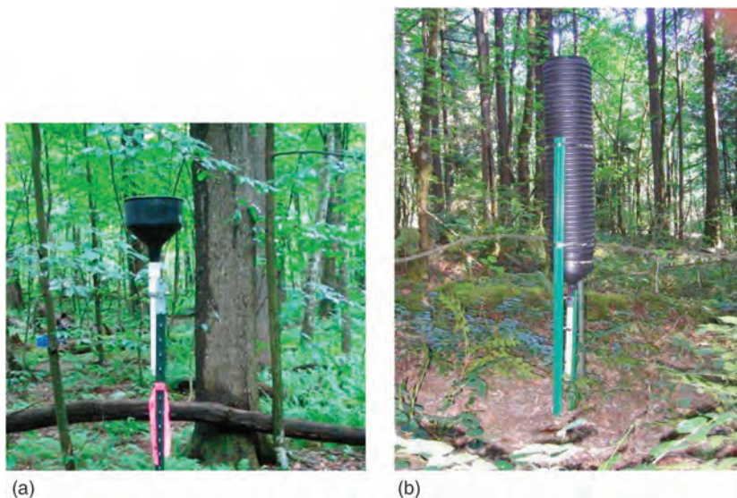
Figure 8.5. A bulk deposition collector using mixed bed (anion and cation) ion exchange resin to collect \text{NH}_4^+ , \text{NO}_3^- , and \text{SO}_4^{2-} in precipitation or throughfall—based on the design described by Fenn and Poeth (2004). The resin columns are usually exchanged after 6 months of field exposure, but in some instances they are changed after 12 months. The collector on the right has a snow tube attached for winter collections.
