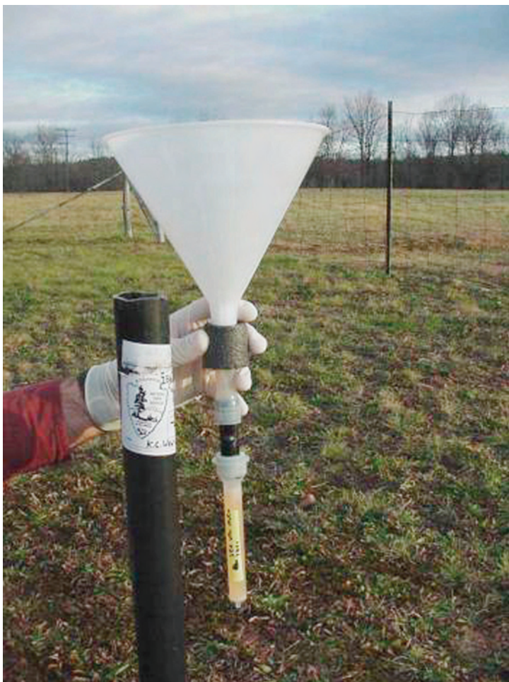
Figure 8.4. A bulk deposition collector using an anion exchange resin column to collect \text{NO}_3^- , \text{SO}_4^{2-} , and \text{Cl}^- in precipitation or throughfall (Simkin et al., 2004). The resin columns are usually exchanged every 6 weeks.
