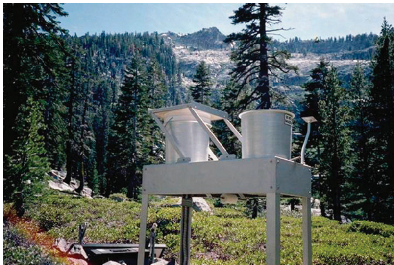
Figure 8.1. Aerochem Metrics model 301 wet/dry bucket collector of the type used in the NADP monitoring network. These collectors are AC or battery powered and are used to collect wet deposition only.
