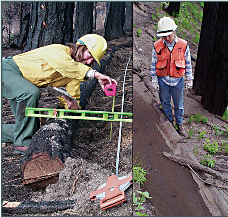
Researchers measure the capacity of a contour-felled log erosion barrier (left) and examine sediment after a high-intensity rainfall event (right).
