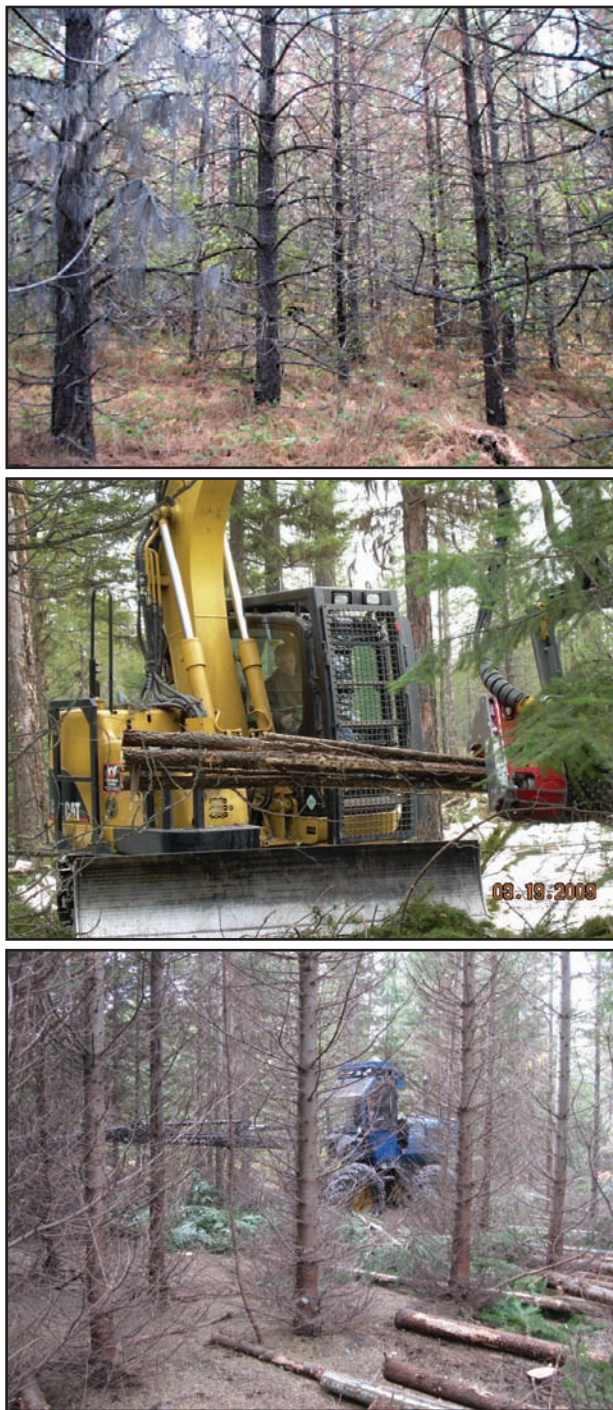
Figure 3 —Young plantation (Templemental Stewardship Project, top) is subjected to variable-density thinning using Cat 314 (middle) and Rottne 2002 (bottom) mini-harvesters (shown working recently in private property areas).
