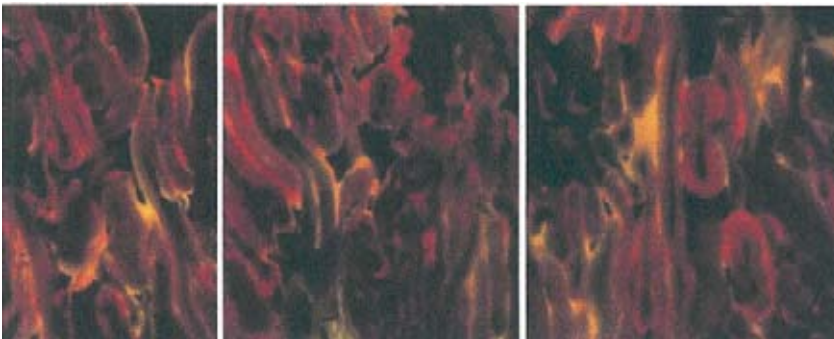
Figure 9. Confocal microscope images of soy-PF infiltration with more adhesive bidding evident between MDF fibres. The specimen was embedded in wax to aid in sectioning.
