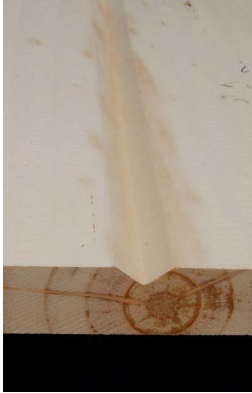
Figure 15. Diffuse extractives bleed from heartwood of radiata pine.
