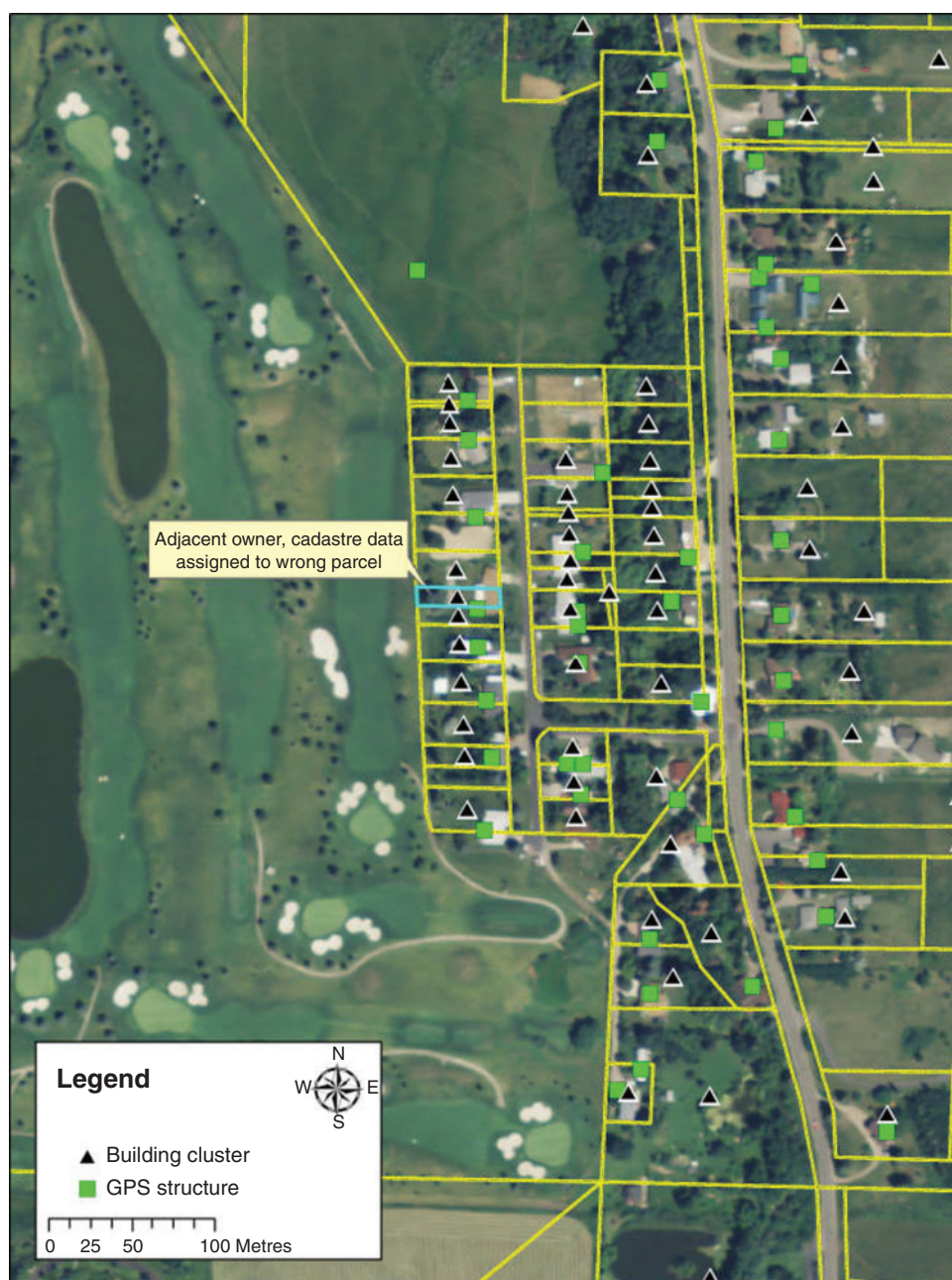
Fig. 5. Adjacent owner: cadastre data assigned to wrong parcel.
