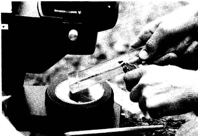
Figure 3.—Shaving an increment core.
