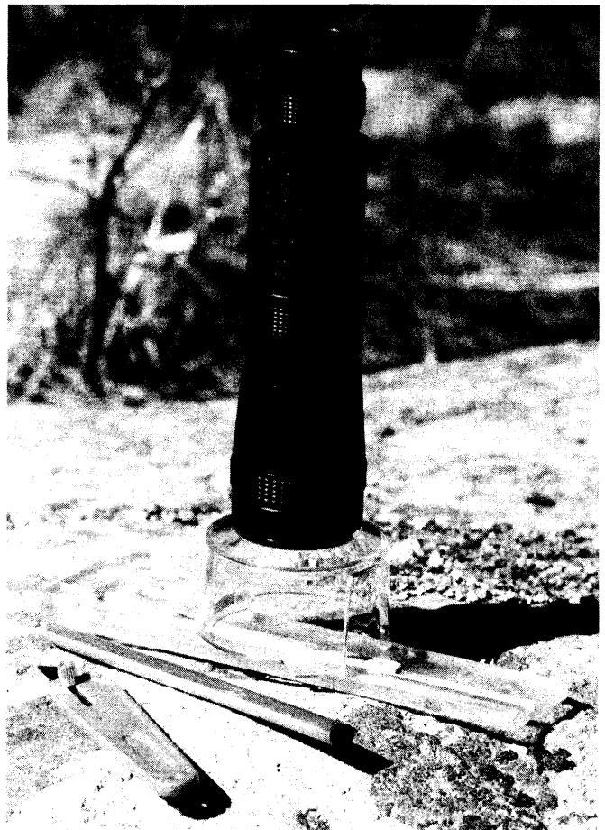
Figure 5.—A variable magnification, lightweight monocular microscope.
