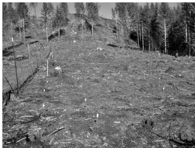
Figure 2. Simulated browse study site with all large slash and residual live trees removed. A 2.4 m (8 ft) fence was constructed around the perimeter of the site, which extended 30.5 cm (12 in) into the soil. The first 0.6 m (2 ft) from the base of the fence was covered in chicken-wire to exclude rodents.
