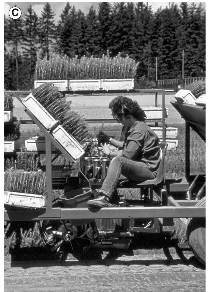
Figure 2. Technology for transplanting has evolved over time from the labor-intensive manual transplanting using boards (A) (Savenac nursery photo archives), to mechanical planting of individual rows (B) (Savenac nursery photo archives), to modern transplanting in multiple rows (C).
