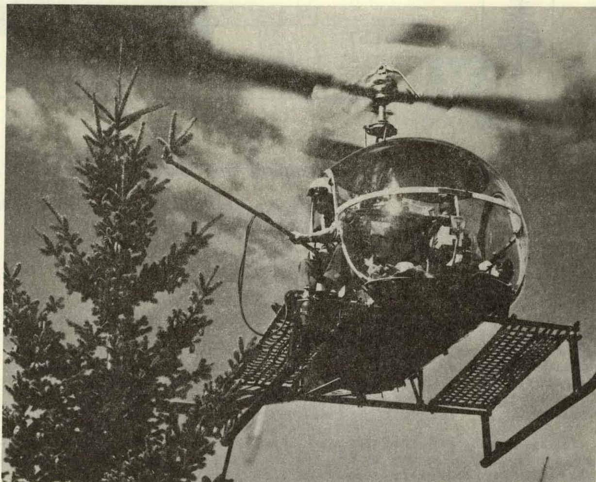
Figure 1.--Helicopter hovers next to the top of a tall Douglas-fir tree while a branchlet is clipped with the newly developed tree pruner to sample foliage.
