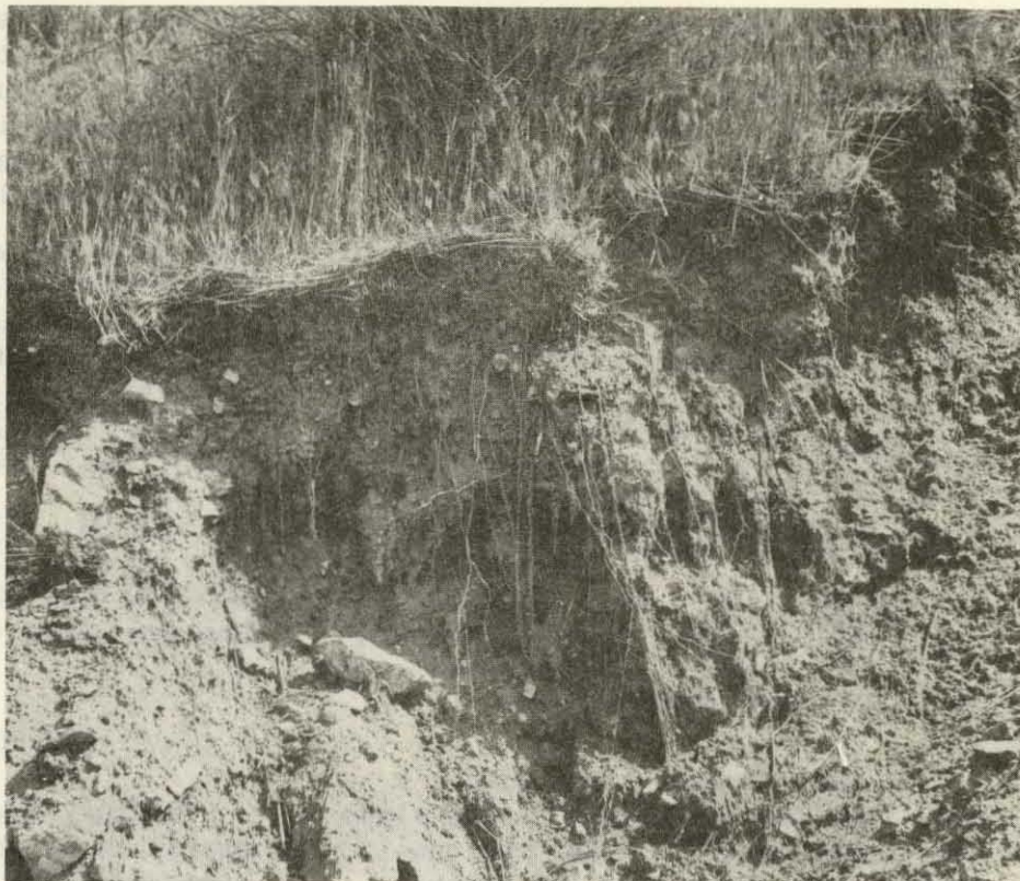
Figure 3.--Type of soil slip in which the shear zone occurs at interface between grass roots and subsoil.
