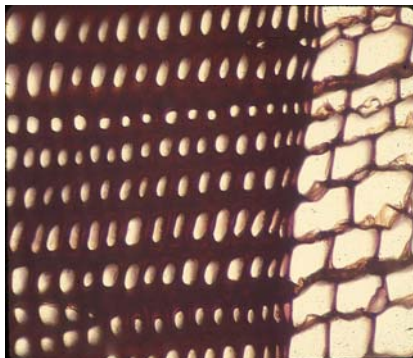
Figure 5 – Heat treated wood showing a darkening and slight cell wall shrinkage.
