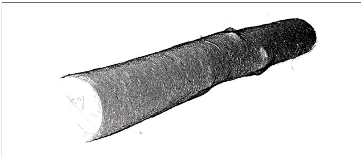
Figure 1.—Dot cloud image of a laser scanned log (Log 2).
