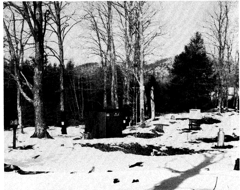
This environment station in a sugarbush is used to monitor solar radiation, soil temperature, sapflow and tree pressure, snow depth, windspeed and direction, soil moisture, humidity, temperature, atmospheric pressure, and precipitation.
