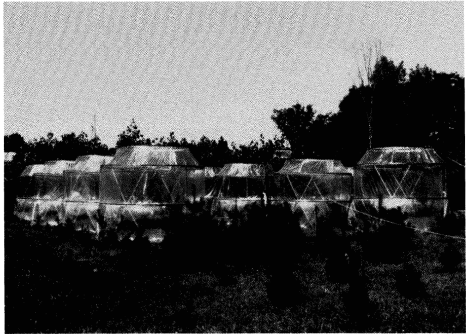
Open-top growth chambers are used to study the impact of air pollutants on tree growth at the Delaware laboratory.
