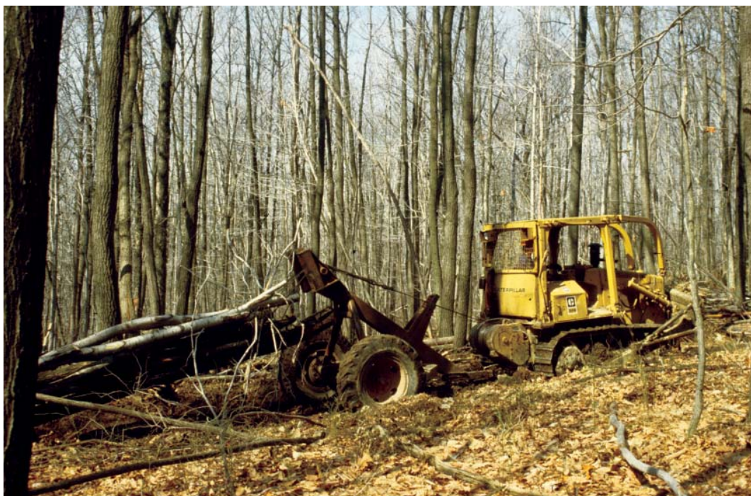
Figure 5.—Harvested trees were pulled from the treatment plots with cable, and skidded out with a Cat® D4 and arch using perimeter roads to minimize damage to residual trees.
