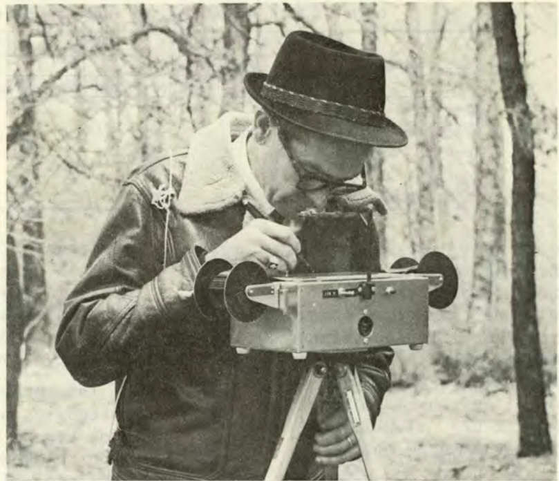
Figure 2.--Portable light was used to view aerial films taken over a flight line. The photo interpreter marked the location of trees on the film.
