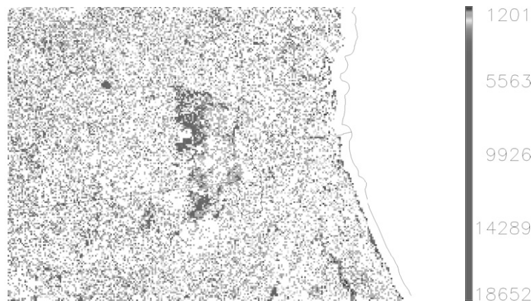
Figure 6: 2006–2008 transition map (values scaled by 1000) for the area around the Okefenokee Swamp on the Georgia-Florida border. Large red areas in the center of the map correspond to fire damage from the Bugaboo scrub fire that burned from April to June of 2007.
