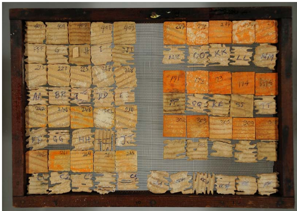
Figure 2A Cross sections of all transverse block-pairs after 4 weeks in test #2. NHA (orange) vs untreated pairs. All numbered blocks = NHA, all letter blocks = untreated choice blocks. From 250-10,000ppms. 6 blocks in lower right [CC1-ff) represent untreated control pairs (3) Blocks are paired: above = NHA treated/ under = untreated: eg402/FFF; 174/SS.
