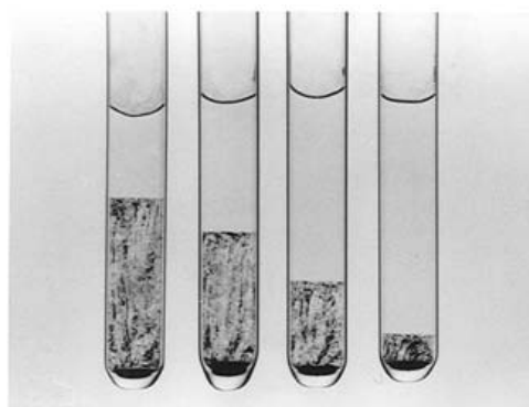
Fig. 14 CNC suspension showing separation into clear isotropic and structured chiral nematic phases as viewed through crossed polarizer. 134 Reprinted with permission from ref. 134 © 1996 American Chemical Society.
