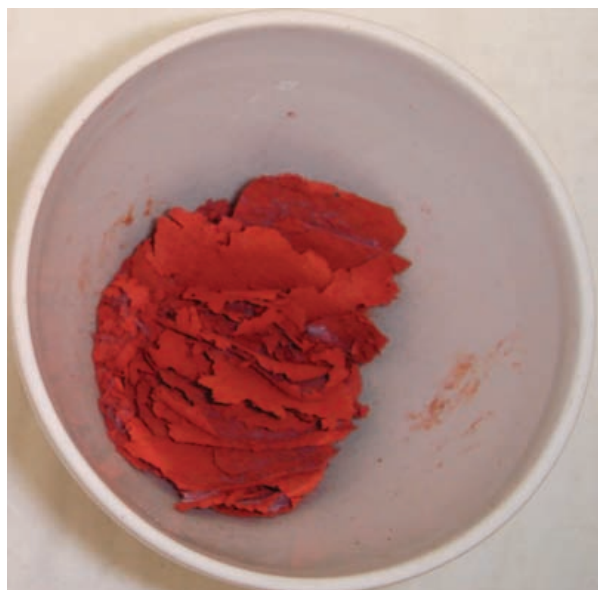
Figure 1. Ash of flotation rejects from a toner printed paper sample.
