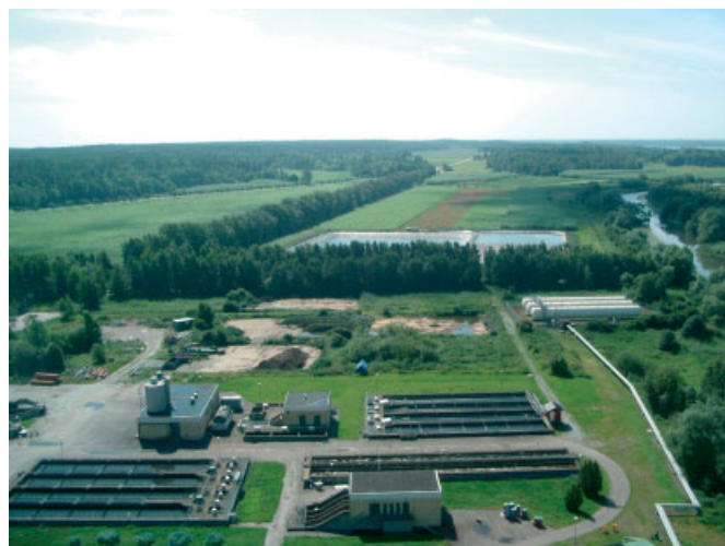
Figure 4. View of the municipal wastewater plant, with water storage ponds and (behind the ponds) the willow fields that are used as vegetation filters. (Photo credit: Pär Aronsson, Swedish Agriculture University.)
