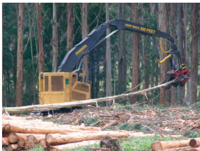
Figure 2. Tigercat tracked harvester delimbing and topping a felled Eucalyptus nitens stem during a streamside harvesting study that utilized Best Management Practices. Note the slash coverage remaining in the harvested area. (© Daniel G. Neary.)
