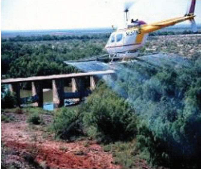
Figure 10. Helicopter mounted with spray system. From Sisneros (1994).
