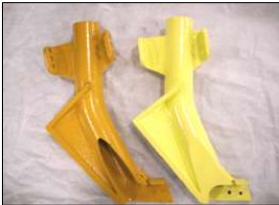
Figure 1. Boot casing. Oblong opening, left, permits seed to fall against disc blade
