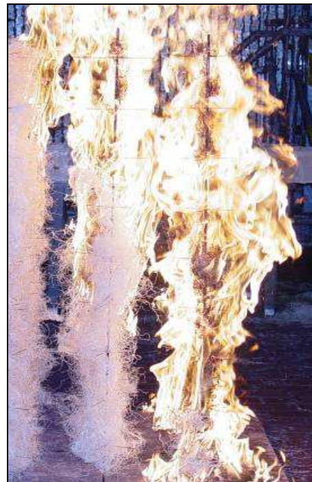
Figure 2 Experimental fire spreading right to left through fine excelsior (shredded Populus spp.). Observations revealed the ignition of adjoining fuels without significant pre-ignition pyrolyzate emissions (clear gaps) and only after flame contact.
