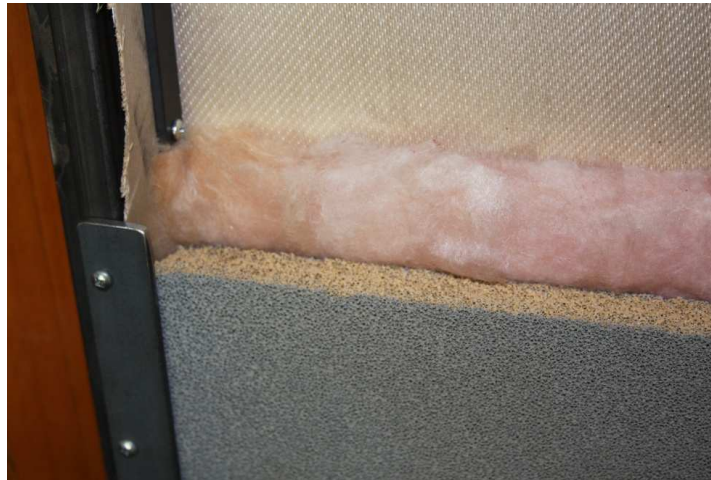
Figure 3. The flame wall burner assembly cross section showing fiberglass cloth (back), fiberglass batting (middle), and porous ceramic plate (front).
