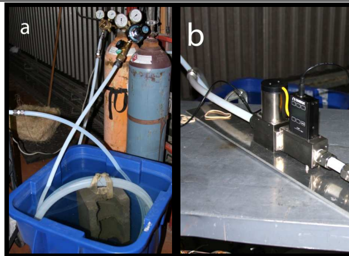
Figure 4. The gas feed system with (a) water bath heat exchanger and (b) Omega Inc. mass flow controller.
