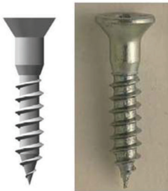
Fig. 6: Actual No. 10 wood screw and mathematical model
