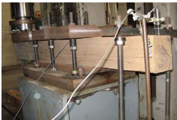
Figure 8: Destructive testing for cantilevered post strength
