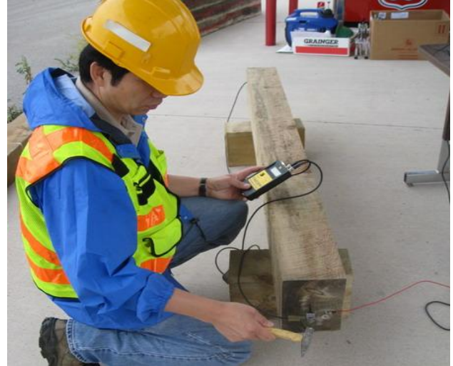
Figure 5: Parallel-to-grain stress wave timing of new posts prior to installation at the Royalton test site
