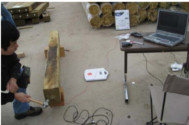
Figure 11: Testing of new posts prior to installation at the Merrimac test site
