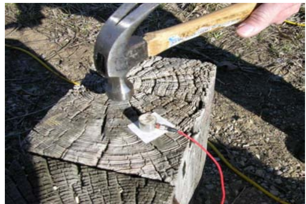
Figure 2: Pulse-echo acoustic testing of an old guardrail post in the field
