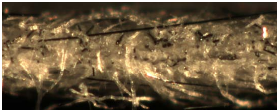
Figure 4. Cross section of a eucalyptus handsheet containing 10% carbon fiber by weight.
