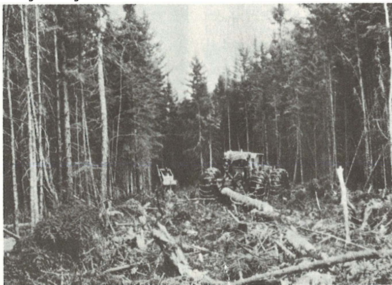
Figure 5.—Large machines can operate in relatively narrow strips. Few residuals are left standing within the strip, and damage to edge trees need not occur.
