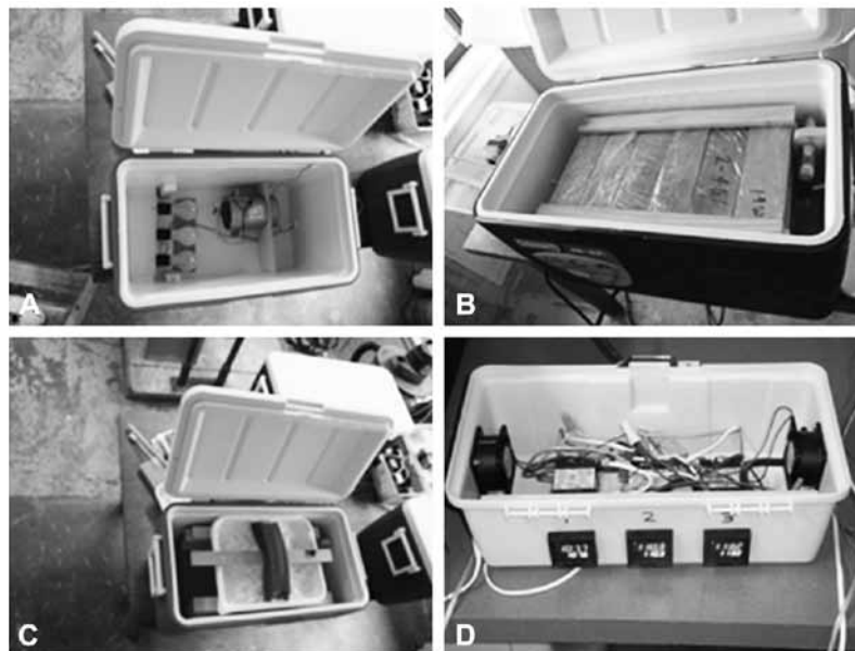
Fig. 1. Conditioning chambers showing incandescent bulbs and fan assemblage (A) loaded with plastic-wrapped samples, with yellow thermometer protruding from a hole in the left side and a data logger on the right side, (B) with a salt pan installed and foam spacer to divert air flow, (C) and control box showing three control assemblies with temperature readouts visible in front (D).
