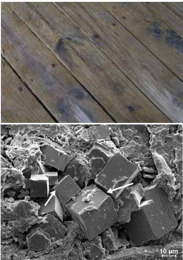
Figure 3. Image of salt damaged deckboards at Isle of Palms Marina (a) and salt crystals (white arrows) located in corresponding sample using Scanning Electron Microscopy (b, 450× magnification).
